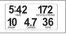
The upper right corner of the display will show the distance you have pedaled, in total revolutions. The display will also show your heart rate when you use the handgrip pulse sensor (see step 5 on page 15).
